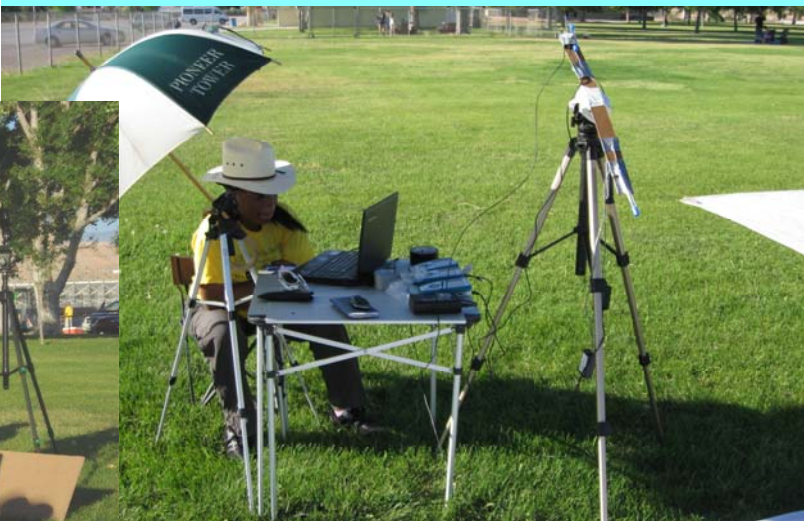
Figure 1. Jackie Sparks mans the laptop recording sky spectra. On the table are Vernier LabQuests connected by wires to sensors to the tripod's wood slat. Three sensors on top face the North Celestial Pole to record temperature, light and sky spectra. One at the bottom was to record shadow bands via light reflected off a white sheet.
