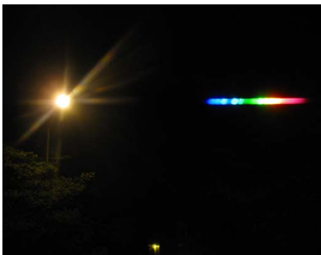
Figure 3. A street light and its spectrum seen with a digital camera and diffraction grating.
